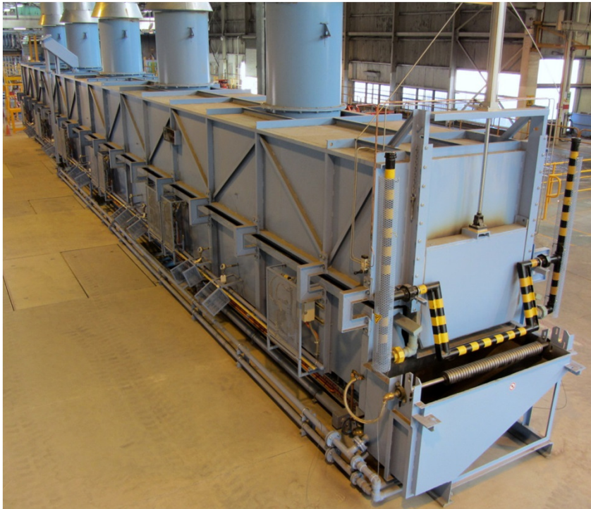
Double Sand Return System with Efficient Air Knife
